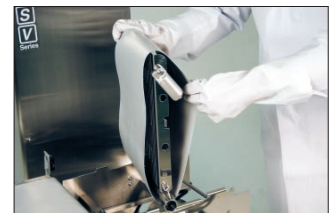
One-touch removal and attachment of conveyor and motor from and to frame
